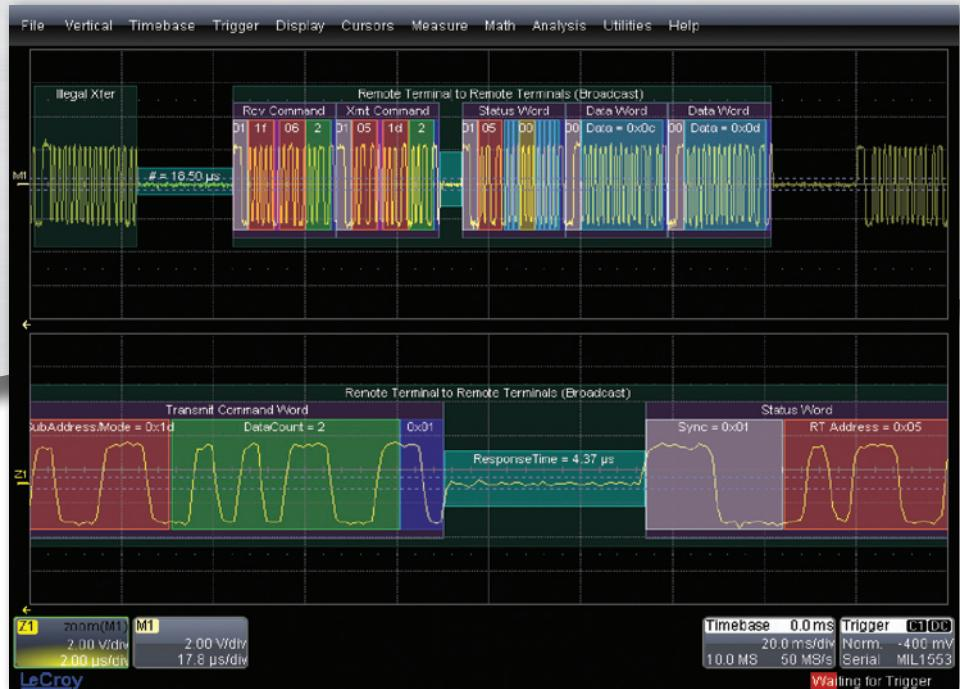
Color-coded overlays help identify the transfer and word type of the 1553 bus messages. Data values are displayed above the waveform that dynamically change depending on the zoom window.
