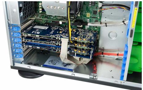
**Item 3:** One of the **streaming options** which consists of a RAID controller and either fast HDD's (for low speed transfer, high storage space) or fast SSD's (for high speed transfer, lower storage space). There are some predefined standard streaming options but other options are also available on request. All predefined options are listed in the order options chapter at the end of the data sheet.
