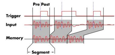
Multiple Recording is ideal for applications where signals arrive in bursts or are generated in a stimulus-response manner. Examples include RADAR, LIDAR, SONAR, Ultrasound, Medical Imaging, RFID, Wireless Communications, Biomechanics, Laser Imaging, Lightening Studies, Nuclear Physics and Radio Astronomy.
