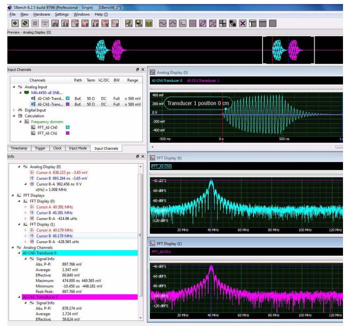
SBench 6 is a powerful and intuitive interactive measurement software. Besides the possibility to commence the measuring task immediately, without programming, SBench 6 combines the setup of hardware, data display, oscilloscope, transient recorder, analysing functions and export functions under one easy-to-use interface. All current Spectrum M2i, M3i and M4i cards are supported.
