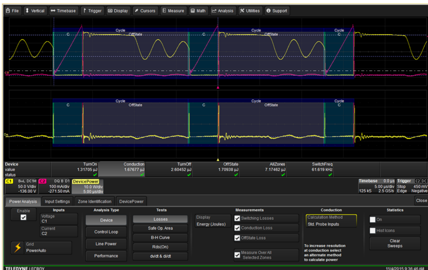
Figure 1: Device Loss measurement parameters include turn-on, conduction, turn-off, off state, all zones, and switching frequency
