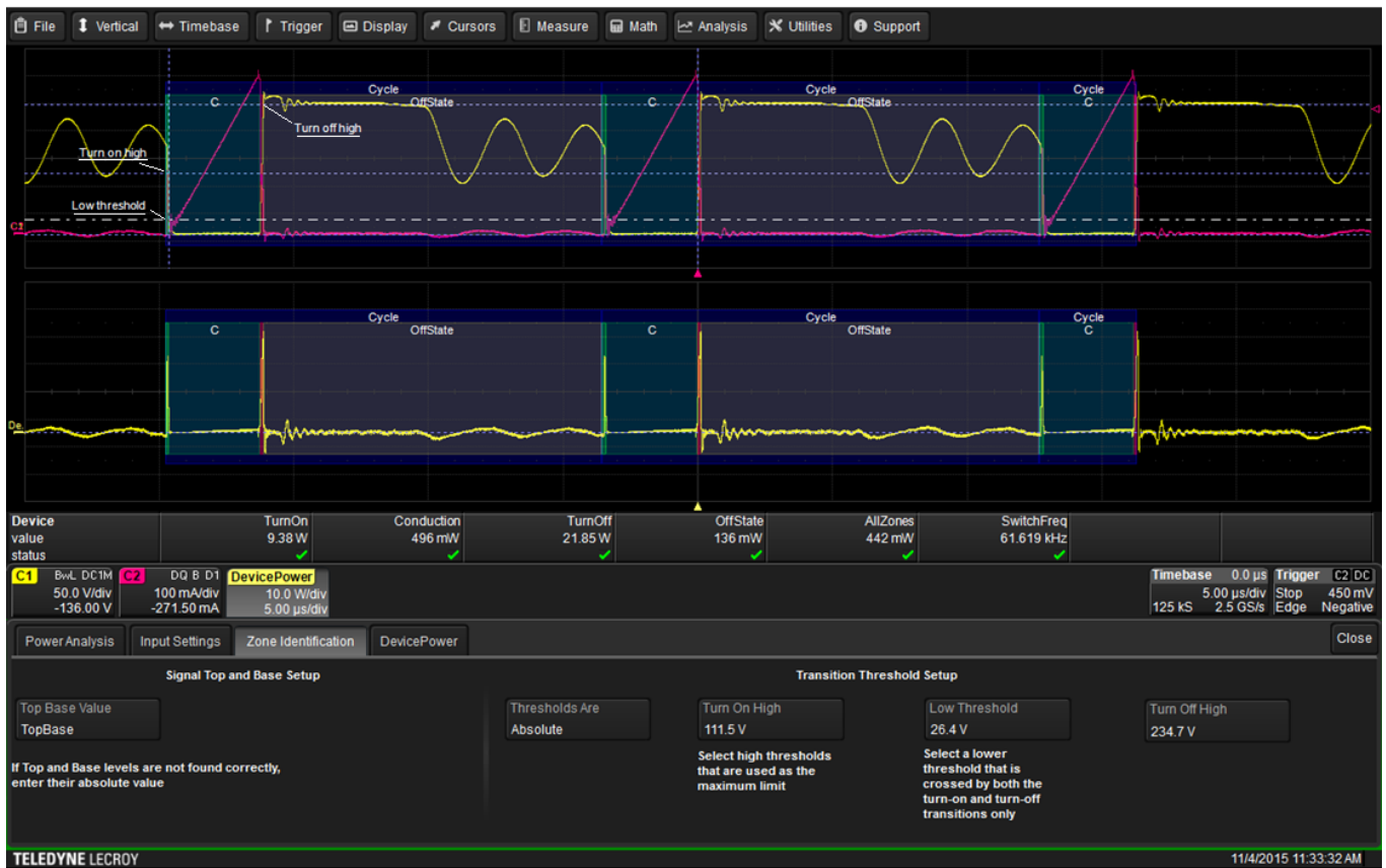
Figure 5: Zone Identification is easily set up by defining the transition threshold levels
